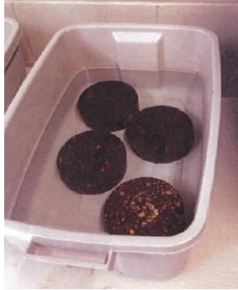
Figure 8. RePlay®-sealed core samples submerged in water at room temperature from Donovan 2013).
